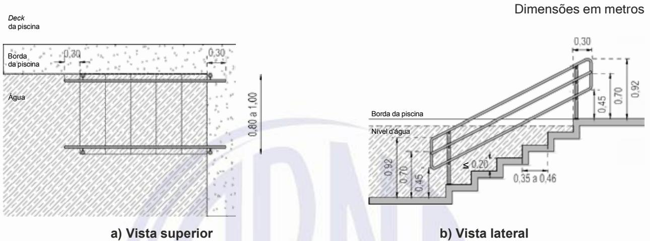
**Figura 150 – Escada submersa**
